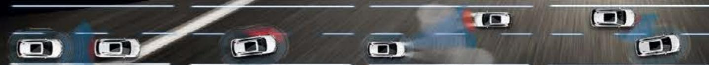
**INTELLIGENT FORWARD EMERGENCY BRAKING:** Intelligent Forward Emergency Braking uses radar technology to monitor the vehicle in front of you, and provide audible & visual warnings prompting the driver to react to avoid a possible frontal collision. Upon driver intervention failure, the vehicle will apply braking to avoid or reduce the severity of the collision.
