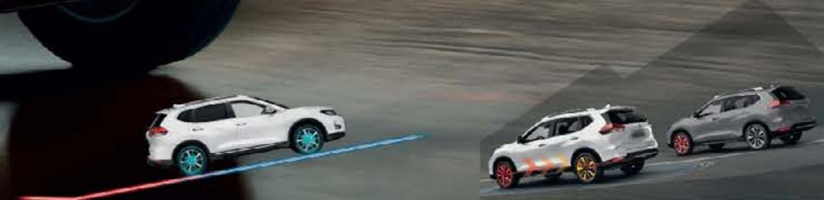
**HILL START ASSIST/AUTO HOLD.** No rolling backwards. With Hill Start Assist, encountering an incline is simple. It applies the brakes to all four wheels to hold the car for 3 seconds, before the drive fed to the wheels releases them. With the Auto Hold function activated, the brakes are held for 3 minutes on any gradient.
