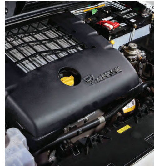
02 - Mahindra's legendary 2.2l mHawk turbo-diesel engine with new 5-speed manual transmission.
