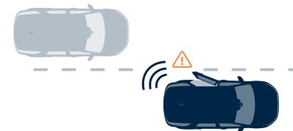
**Clear Exit Monitor** helps rear passengers to exit the vehicle safely by providing an alert of approaching hazards via a small warning light on the door handle.
