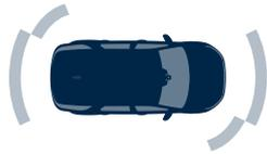
**Front and Rear Parking Aid** uses sensors located in the front and rear bumpers which will help make manoeuvring that little bit easier.
