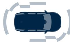
**360° Parking Aid** uses sensors located around the vehicle to indicate how close you are to obstacles via the Touchscreen display and audio feedback.
