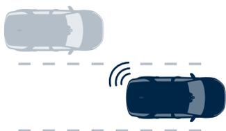
**Blind Spot Assist** can help prevent collisions. If your vehicle detects another car in your blind spot when starting to change lanes, a warning light illuminates in the corresponding door mirror. Corrective torque is applied to the steering wheel, encouraging you to guide your vehicle away.
