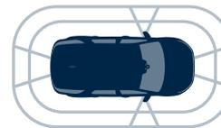
**360° Surround Camera\*** incorporates ClearSight Ground View, as well as Junction and Kerb View technology, to provide a full 360° bird's-eye view of the vehicle on the Touchscreen, giving you the confidence to manoeuvre safely.
