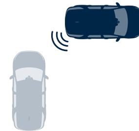
**Rear Traffic Monitor** helps when reversing with an obstructed view by warning you of vehicles, pedestrians or other hazards approaching either side of your vehicle.
