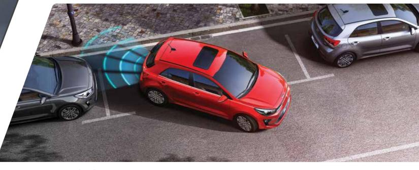
**Parking Distance Warning (PDW) \*** For utmost confidence and peace of mind when maneuvering into and out of tight parking spaces, PDW uses ultrasonic sensors mounted on the rear bumpers to warn you of any nearby obstacles.
