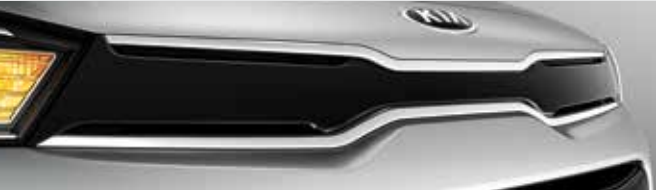
Radiator Grille The iconic Kia radiator grille is completely restyled. Most of the airflow used for cooling enters through the lower intake.
