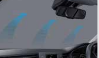
Auto Defog System The auto defogger detects mist on the windshield, and automatically deploys the fans to clear the glass rapidly. Only available on the TEC model.
