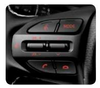
Audio Remote Controls Buttons mounted on the steering wheel let you adjust audio functions while your eyes stay on the road.
