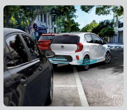
**Rear Park Distance Control** You're lucky to find a parking spot in the city, and rear park distance control can help you reverse with confidence. Using sensors, it beeps faster, then continuously as you get closer to an obstruction.
