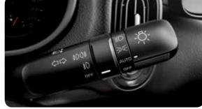
Auto Light Control Set the stalk ring to 'Auto' and the front and rear lights will turn on or off automatically depending on lighting conditions.
