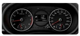
**2.6-inch mono-LCD** Get tyre pressure alerts and other essential vehicle and trip information at a glance with the mono LCD located between the instrument dials.
