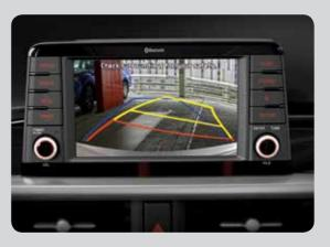
**Rear-view camera with dynamic guidelines** Using a waterproof rear camera and the 7-inch dash display, the rear-view camera projects dynamic guidelines onto the image to recommend a path as the driver reverses. SMART models only.
