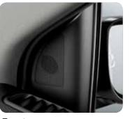
**Tweeters** Tweeter speakers at each end of the dashboard help bring out the high frequencies of the audio signal.
