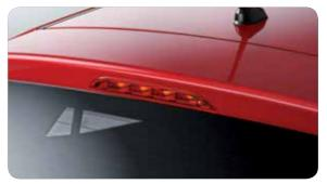
High-mounted Stop Lamp Located on the subtle spoiler above the rear window, the lamp safely alerts drivers behind you when you're braking.
