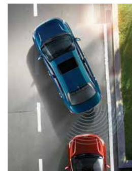
Parking distance warning-reverse Using sonar technology, this system warns you when coming close to objects while backing into parking spots.
