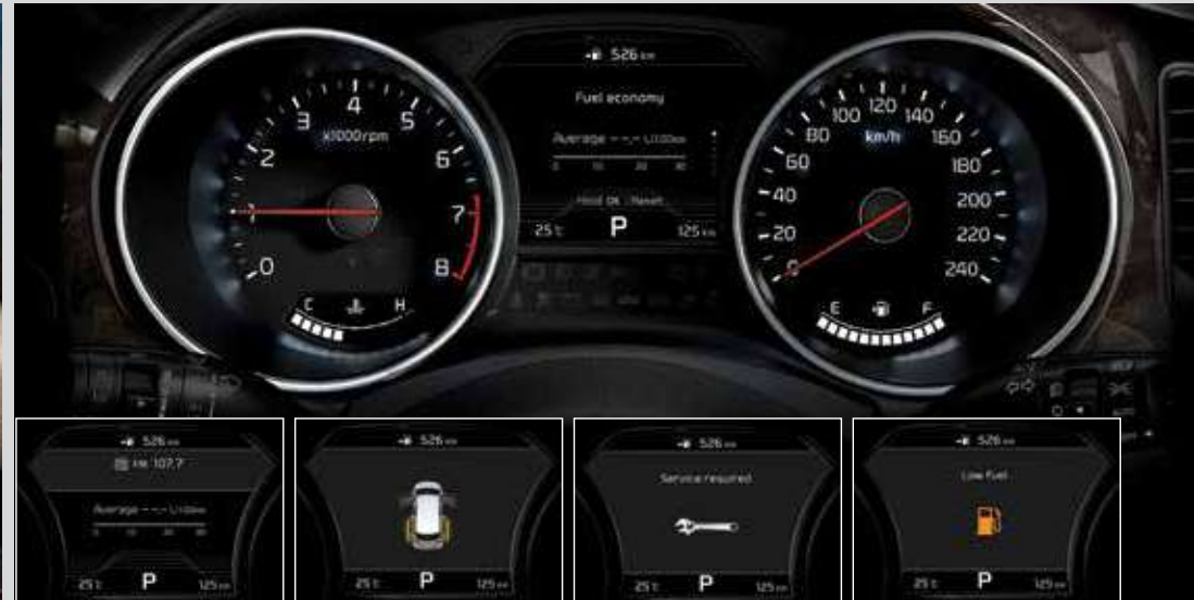
Supervision cluster (7" colour TFT LCD) A high-visibility display located in the centre gauge cluster provides useful, on-demand trip computer information graphics such as distance to empty, average and instant fuel consumption and outside temperature. SXL model only.
