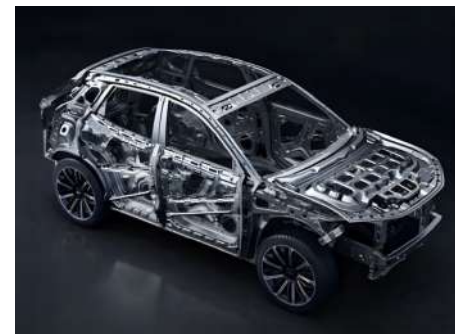
SAFE BODY STRUCTURE 85% HIGH-STRENGTH STEEL
