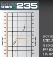
6-cylinder Isuzu SiTEC Series III 235 is specified on the FRR 600 FSR and FTS ranges. It delivers 176kW and an impressive 706Nm torque.
