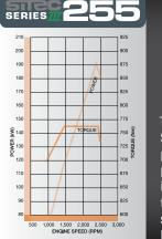
The Isuzu SiTEC Series III 255 produces 191kW power and impressive 761Nm torque and is standard on FRD/ FSD S models.
