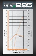
The Isuzu SiTEC Series III 295 produces 221kW power and 981Nm torque and is standard on all FV models.
