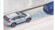
The ACC system is designed to keep a set speed and set the following interval behind a vehicle detected ahead of yours, including the ability to start and stop the vehicle with the flow of traffic.
