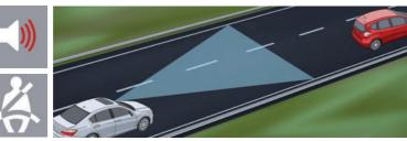
Primary warning: When there's a risk of collision ahead or the distance between the two vehicles is too short, the alarm sounds and the word BRAKE appears on the i-MID (intelligent-Multi-Information Display). This alerts the driver to take action in order to avoid collision.
