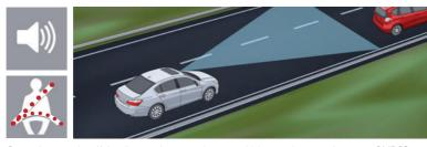
Secondary warning: If the distance between the two vehicles continues to decrease, CMBS® applies light braking and the seatbelt E-pretensioners in the driver's side gently pull two or three times. At this point the E-pretensioners pull the seatbelts with enough force to properly restrain you and your front passenger, giving you time to react and avoid a collision.
